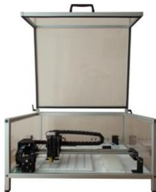
Prints up to 400 (20620) samples in each well of 96-well plate or up to 30K samples on glass slides 1"x3"
