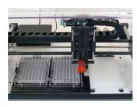
Prints DNA, oligonucleotides, proteins, bacterial clones and other materials with low cross contamination using metal-ceramic capillary pins Xtend.
